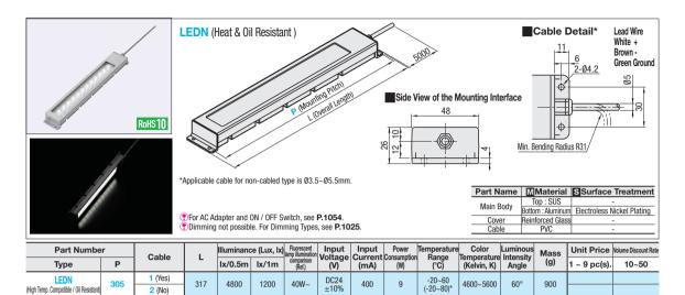
\*When using in 60°C ~ 80°C environment, be sure to mount on 50cm square and 2mm thick metal plate.
