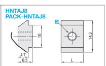
•Overall length is shorter than Pre-Assembly Insertion Nuts HNTT. Suitable for installing sensors or other con
