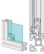
Holes are tapped on a bracket for cover mounting.
