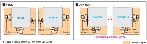
Three open sides are needed for Feed Knobs and Clamps · Sufficient space must be retained for adjustment.
