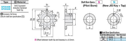
For double pitch chain idlers, see E P.1552. Part Number Shaft Bore Dia. Unit Price Shaft Bon Mass Specification (DH8) Operating Teeth Х Dρ Do l н Specs. (kg) 0.64 78 23 84 60 1/2 10 1/2 86.17 92 69 0.93 **SP2040B** 25 7.2 77 94.15 100 0.99 11 1/2 N 102.14 108 63 1.06 1/2 14 97.78 105 19 1/2 1.1 9 s 10 1/2 107.72 115 1.62 **SP2050B** 73 28 8.7 8 1/2 117.68 125 1.74
