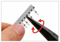
Individual comb-style jumper bars are created by breaking out jumper contacts (starting with 3-way).
