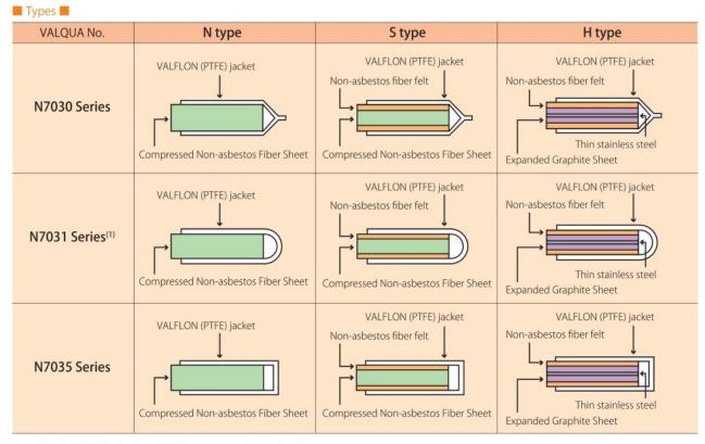
Note (1) No.N7031 Series has a PTFE outer cover with one lap joint.
