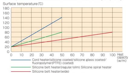
The temperature in the table is the temperature obtained by measuring a single heater in a horizontal state in the air at room temperature of 20°C. Add or subtract the actual ambient temperature.
