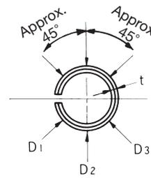
Slot width "C" should be chosen safe from closely contact when spring pins are inserted. (exception: both ends of spring pins)
