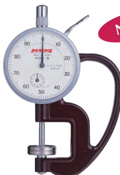
G-20 Graduation: 0.01mm Range: 0~10mm
