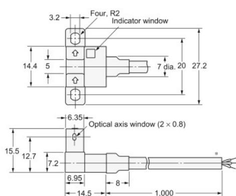
\* Vinyl-insulated round cable of 3.5 dia., 3 cores,
