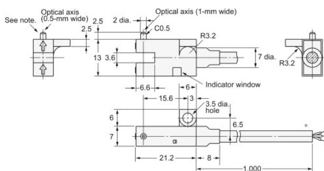
\* Vinyl-insulated round cable of 3.5 dia., 3 cores,
