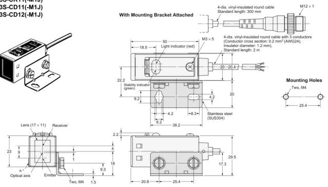
Note: Models numbers for Through-beam Sensors (E3S-CT61(-M1J)) are for sets that include both the Emitter and Receiver. The model number of the Emitter is expressed by adding "-L" to the set model number (example: E3S-CT61-L 2M), the model number of the Receiver, by adding "-D" (example: E3S-CT61-D 2M.) Refer to Ordering Information to confirm model numbers for Emitter and Receivers.
