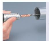
Wire lapping tools are made from banded piano wire. Ideal for burr removal and finishing of metals and plastics. They are also suited to polishing with abrasive compounds.
