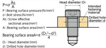
Head Diameter and Screw Effective Cross-sectional Area
