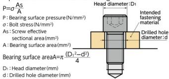
Head Diameter and Screw Effective Cross-sectional Area
