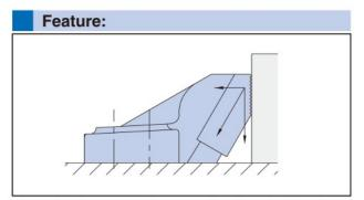
These backstops work to provide downholding force and prevent part lift.
