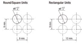
Note: Determine mounting centers to ensure easy operation.
