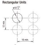
Determine mounting centers to ensure easy operation.
