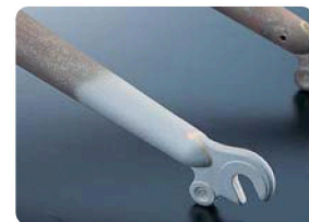
Surface preparation before painting (#120 abrasive used)
