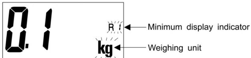
2. Release the **Range** key. Press the **Range** key again to select a minimum display.
